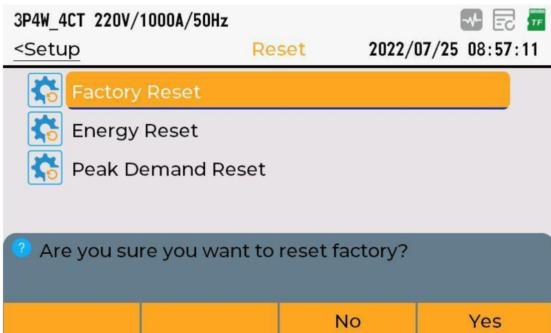
(Figure 6-32 Operation Confirmation Interface)
